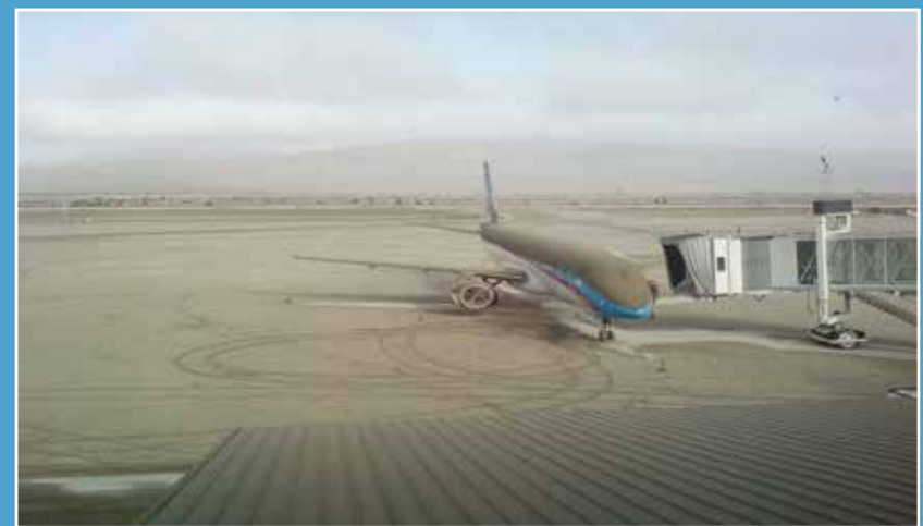
5-10 mm of ash fall at San Carlos de Bariloche International Airport in Bariloche, Argentina, following the June 2011 eruption of Peyuhue Cordon-Caulle volcano in Chile. The airport closed for 31 days due to the on-going ash falls, remobilisation of ash and cleanup.
